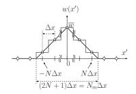
Applying multiple moving average is equivalent to moving average with which central weight is larger than neighboring points.
